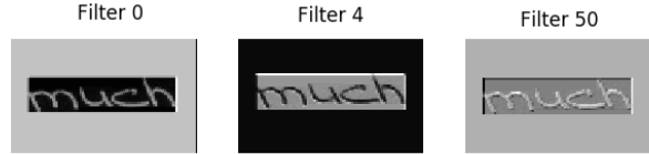
Figure 3. These are the filters from the first convolutional layer of the RESNET-18 word segmentation model with the example word "much"
