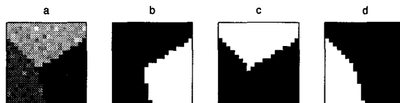
Figure 4: (a) A synthetic image showing three image patches forming a junction. Image intensity varies from 0 to 1, and Gaussian noise with \sigma = 0.1 is added. (b)-(d) shows the top three components of the partition.
