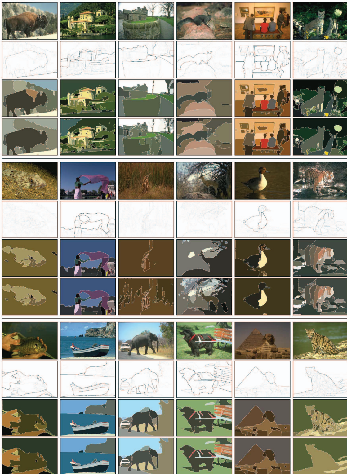
Fig. 16. Additional hierarchical segmentation results on the BSDS500. From top to bottom: Image, UCM produced by gPb-owt-ucm , and ODS and OIS segmentations. All images are from the test set.
