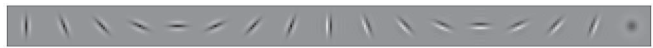
Fig. 5. Filters for creating textons. We use eight oriented even and odd symmetric Gaussian derivative filters and a center surround (difference of Gaussians) filter.
