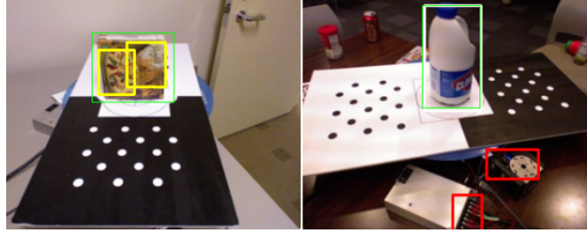
Figure 2. Examples of detection with the baseline method and threshold of 0.97. Red and yellow indicate false positives, white indicates true positive, and the green rectangle is the ground truth bounding box of the object.
