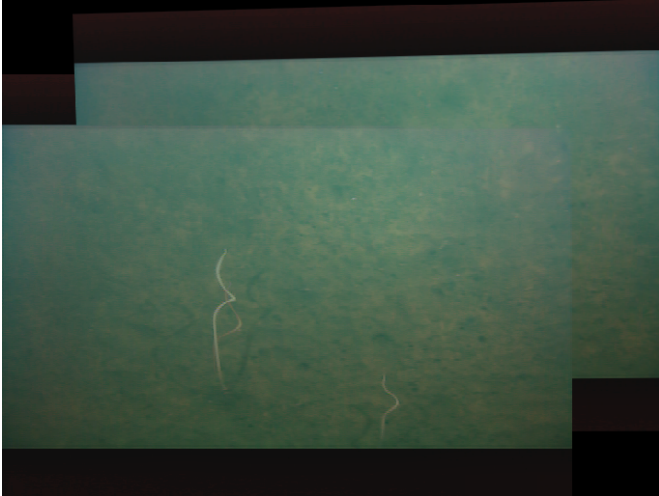
Figure 2. The RANSAC algorithm rejected the false positive matches, yielding a good transformation model between the two images in figure 1.
