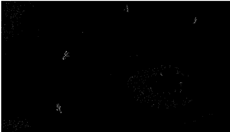
Figure 2. The foreground mask found using OpenCV's Mixture of Gaussians model.
