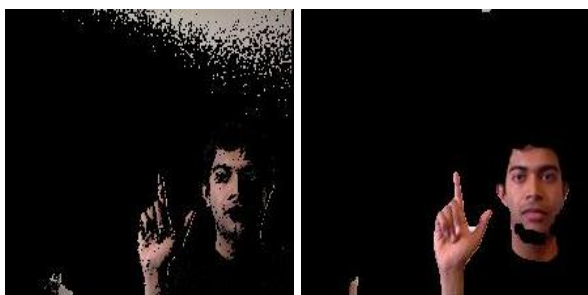
Figure 4: (Left) Skin detected using Gaussian model, (Right) Skin detected using YIQ and YUV color spaces
