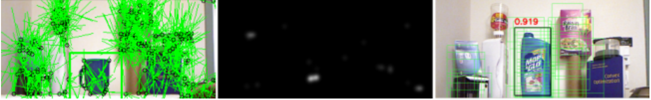
Figure 2. Left: Visualization of Hough voting scheme. Every black circle is a weakly-detected part, and green lines indicate votes. The green lines meeting at the center of the tea cup give rise to a noticeable peak in the response map for that object ( Center ). Right: Visualization of the root filter template matching. Proposed locations are shown in green and filtered further. The black rectangle is a true positive match obtained from subsequent filtering.
