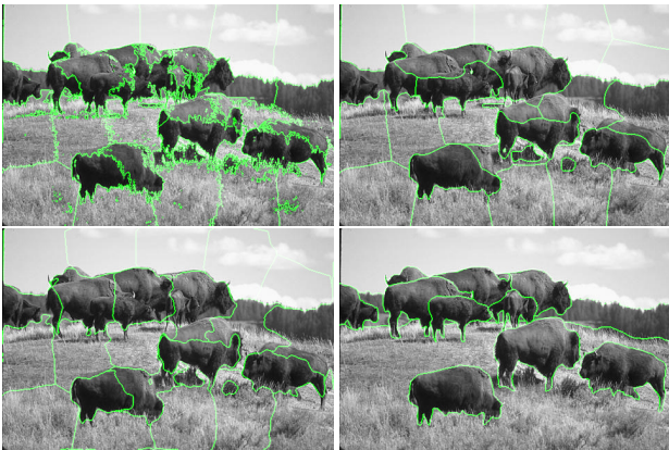
Figure 3. The top two images show the resulting segmentation after applying k -means directly to the original image and to the TVD smoothed image. The latter is much more visually appealing. To show that arbitrary smoothing will not necessarily solve the problem, the bottom left image depicts the results from applying a Gaussian filter to the image. Finally, the bottom right image depicts the ground truth (24 segments) as labeled by a human.
