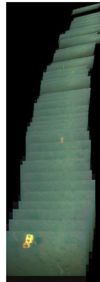
Figure 6. The affine model also falls victim to the distortion seen in the rotation model, though its manifestation is different. Each successive frame suffers from a greater degree of skew, rotation, and scaling.
