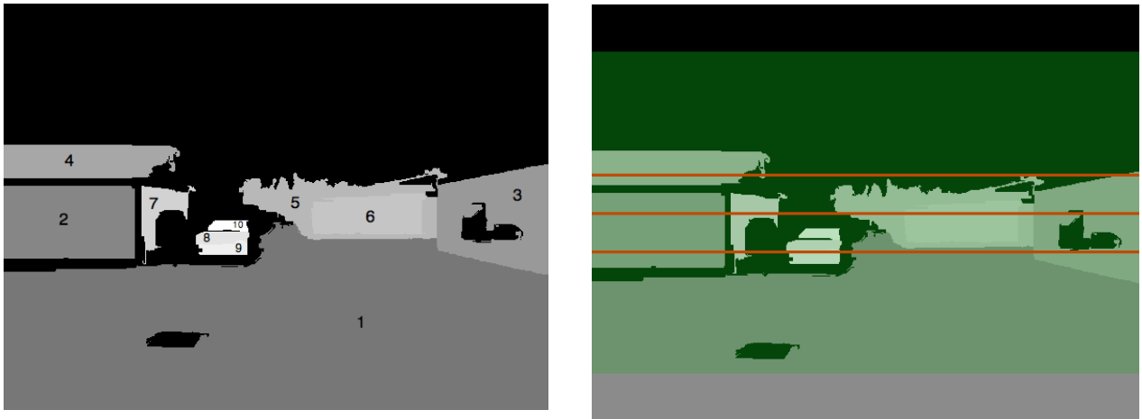
Figure 5 – (a) Segments identified as planes, (b) Horizon lines for various assumptions on viewing angle
