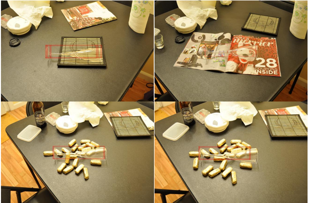
Figure 7. Even in the presence of various degrees of background clutter, template matching managed to find the transparent glass. In the last two images, the scales of the glasses are different, but both objects were detected successfully, suggesting that this method is robust to slight changes in scale as well.
