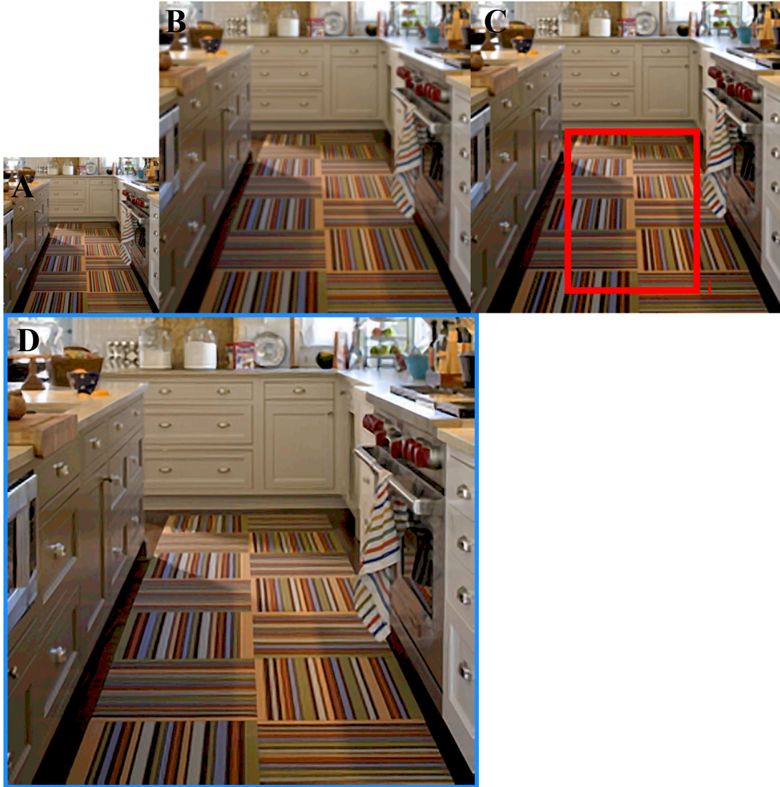
Figure 6: Kitchen (man-made pattern) a) Original image (1x) b) Bilinear (2x): lots of blurriness c) Yue (2x): clear, but floor pattern contains aliasing shown by (i) d) Glasner (3x): clear, less aliasing
