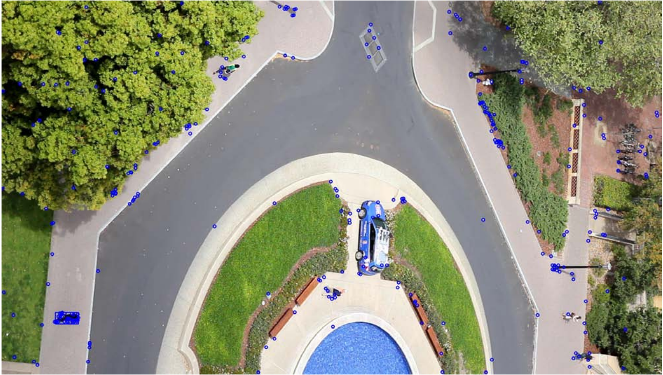
Figure 7: Object recognition for pedestrian on one frame using SIFT descriptor and classifier. The blue circles are key points. We can see that it recognize only one pedestrian on the bottom left, which that specific pedestrian belongs to labeled training data. It does not recognize the other pedestrians.
