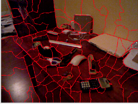
Figure 8: Laptop, ruler and calculator merge with table-top but laptop is separate from wall.
