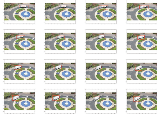
Figure 9. Another classification testing result of multiple classifications. In this case, truck is successfully classified from the cart object and the classification are correct for all the frames. Because this video clips is longer than others (due to the low speed of the truck), the sample is one frame out of each 10 tested frames.
