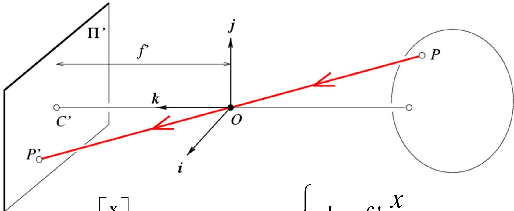
$$P = \begin{bmatrix} x \\ y \\ z \end{bmatrix} \rightarrow P' = \begin{bmatrix} x' \\ y' \end{bmatrix} \quad \left\{ \begin{array}{l} x' = f' \frac{x}{z} \\ y' = f' \frac{y}{z} \end{array} \right.$$
