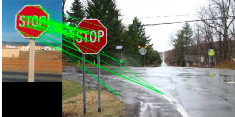
Figure 4: Sample Output, showing training image, keypoint correspondences and resulting bounding box
