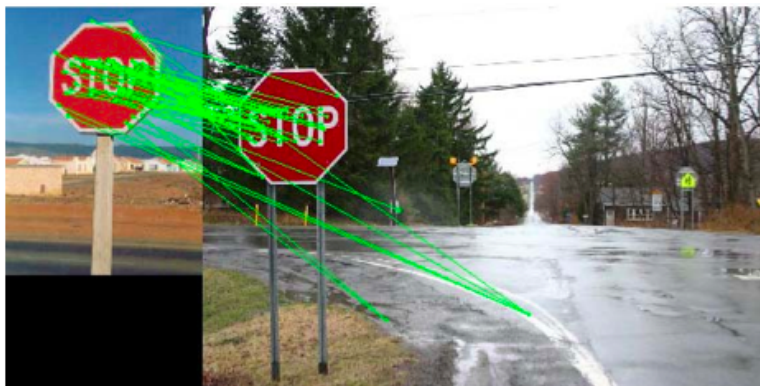
Figure 5: Sample Output, showing training image and keypoint correspondences.
