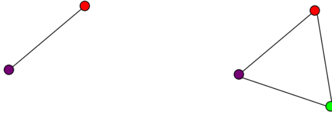
Figure 1: Mixing two lights produces colors that lie along a straight line in color space. Mixing three lights produces colors that lie within the triangle they define in color space.
