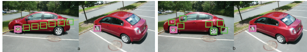
Figure 4. Image pairs show the candidate part correspondences (green boxes) and the correct one (red box) in the left figure across nearby viewpoints given a part (red box) in the right figure. In the left image pair, our full model enforces the candidate part correspondences in the left figure to belong to the epipolar line (the yellow line). In the right image pair, a model without the epipolar constraints yield arbitrary part correspondence locations in the left figure. This, in turn, increases the likelihood of obtaining erroneous part detections and correspondences, such as the back wheel of the car.
